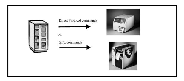
When the host software cannot be changed, a computer must be connected between the host and the command language based printer. A computer software application converts the host data into a data string that the printer will understand:
