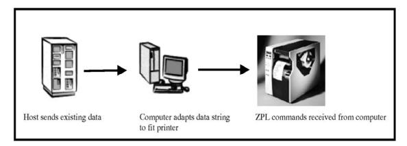
Using Fingerprint, the printer is instead programmed to receive the host data and to pick the appropriate information from the data string for printing:
