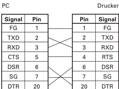
9-Pin – 25-Pin-Kabel
