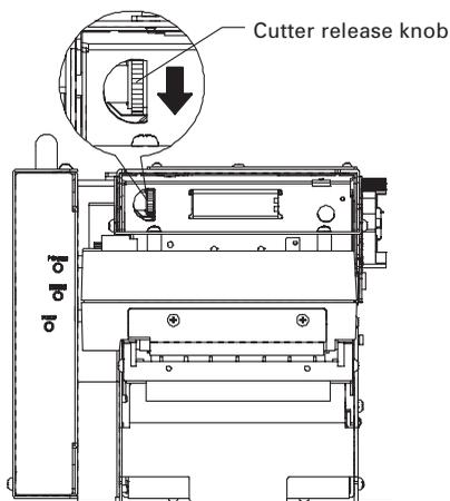
4. When the control box is set apart from the printer, turn the cross hole shown in the figure in the arrow direction to restore the blade.
